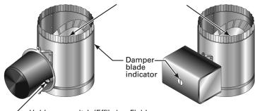
Hold-open switch (Effikal or Field Controls only) — Install vent damper so that switch is visible and accessible to user.
